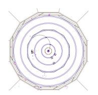
Losses of clusters for < 2 GeV charged particles due to **5 T** field and increased inner radius to 2.1 m
